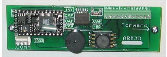
**Step 2:** Solder in all 4 capacitors (0.1uF) as seen in the picture labeled CAP. Polarity (positive and negative leads) doesn't matter in these capacitors.
